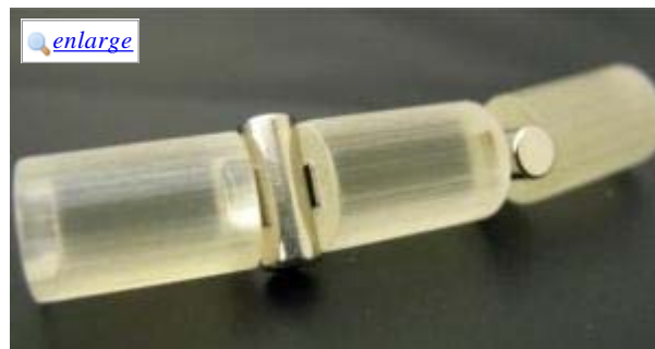
A model of a self-assembling stomach robot: a magnetic mechanism connects three modules together via intermediate linkages. (Credit: Image courtesy of ETH Zurich)
